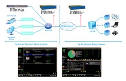
Integrated in the network with the DVStorIP-Gen, designed to simulate a fully operational IP video delivery headend, the duo makes a complete video over IP quality assurance solution - monitoring all MPTS and/or SPTS streams on a fully loaded GigE link, allowing all layer coverage: video content, TS and IP layers, impairments on the fly and many more.
