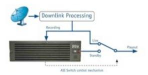
One vital feature of the DVStor<sup>2</sup> as a disaster recovery system lies in the ability to detect loss of signal on input streams. As DVStor<sup>2</sup> continually records and analyzes transport streams, it can trigger the play out of the recorded transport stream over either the IP or the optional ASI port upon detecting an input failure.
