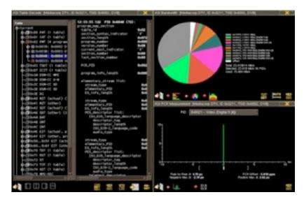
Other features include video thumbnails for MPEG-2 and H.264 video streams in SD and HD for confidence monitoring, On-air Content Validation (OCV) and DVB-H options. OCV allows automatic identification of discrepancies between the expected baseline and actual broadcast content.
