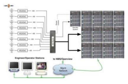
DVStor<sup>2</sup> eliminates the need for costly external storage by offering maximum compression. Video services can be transcoded in-place without modifying the transport stream structure. Efficient storage space is further achieved as DVStor<sup>2</sup> notes the presence of null packets in the stream, removes them when recording and reinsert them on playback.
