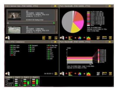
Another feature is the real-time transport stream monitoring. Tests include transport stream health check, bandwidth of service and individual PIDs, PCR jitter, automatic On-Air Content Validation, EIT display monitoring and stream capture.
