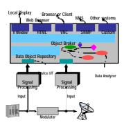
DVStation employs a multi-process architecture, dividing tasks between user/program interfacing and data collection, correlation, and storage.
