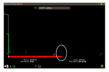
Since the transport stream was automatically captured at the time of the error, the support engineer can quickly inspect the captured file for further analysis. Thus saving time since it is no longer necessary to scroll through huge amounts of data looking for the problem.
