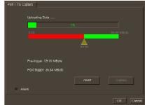
trigger means that data acquisition starts at the exact trigger point. Setting a 100% trigger results in all the data *leading up to* the trigger point – essentially similar to the *black box* flight data recorder used on commercial aircraft, showing you everything leading up to the crash.
