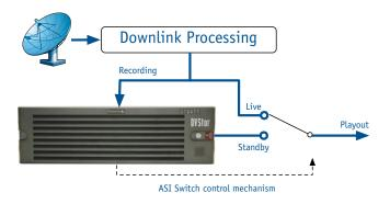
When installed in a live network, the DVStor<sup>2</sup> has three operating states.
